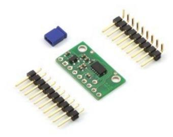
A 10×1 strip of 0.1" header pins, a 9×1 strip of 0.1" right-angle header pins and one shorting block.
