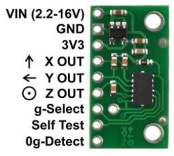
To power the three-axis accelerometer, connect 2.2-16 V battery or power supply to the VIN pin. Note that this part does not have 5V-tolerant pins, so **external components (such as voltage dividers) are required when interfacing the board's g-Select and Self Test pins with 5V systems**. Connections to the g-Select and Self Test pins are optional; the board will work with these pins disconnected.
